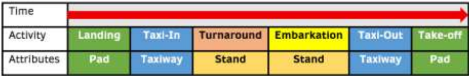
Figure 5. Operation of vertiport, simplified for one aircraft.
