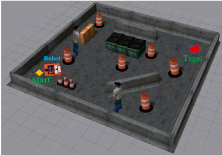
Figure 8. Path planning simulation environment for mobile robots in ROS-Gazebo.
