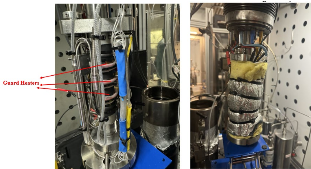
Figure 3. Viton sleeved high-pressure thermal conductivity measurement stacked setup with embedded reference discs, thermocouples, and heater wiring (left) and thermal insulated stacked setup (right).
