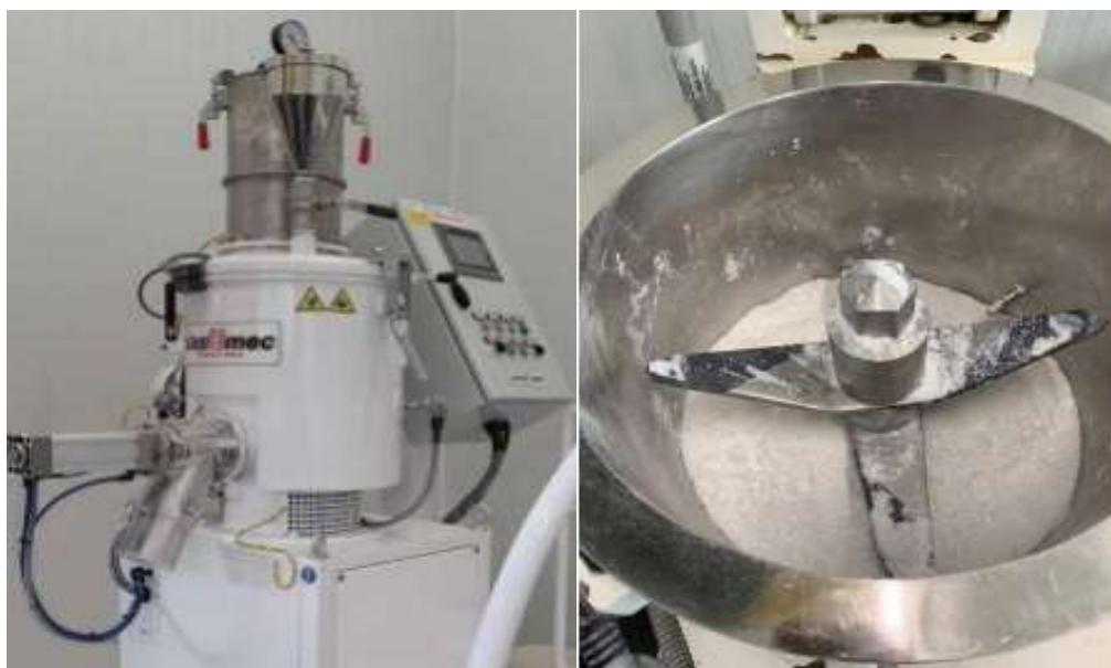
Figure 2. Turbo-mixer for the adsorption process of natural bioactive agents onto silica.
