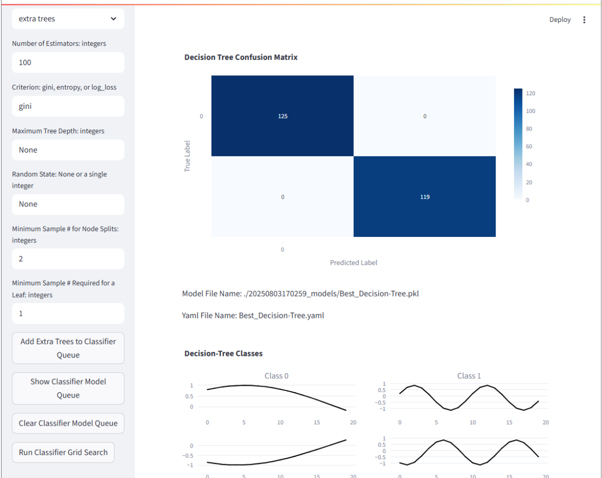
Figure 7. Classification Page is where classification algorithms may be created and queued to run on a loaded dataset. Multiple inputs for each hyperparameter of multiple models may be created and run through a grid search. The best model of each type place in the queue will have results displayed. Here, a confusion matrix and the first three samples of each class are displayed. Note that plots in black are correctly classified and those in red are incorrectly classified.
