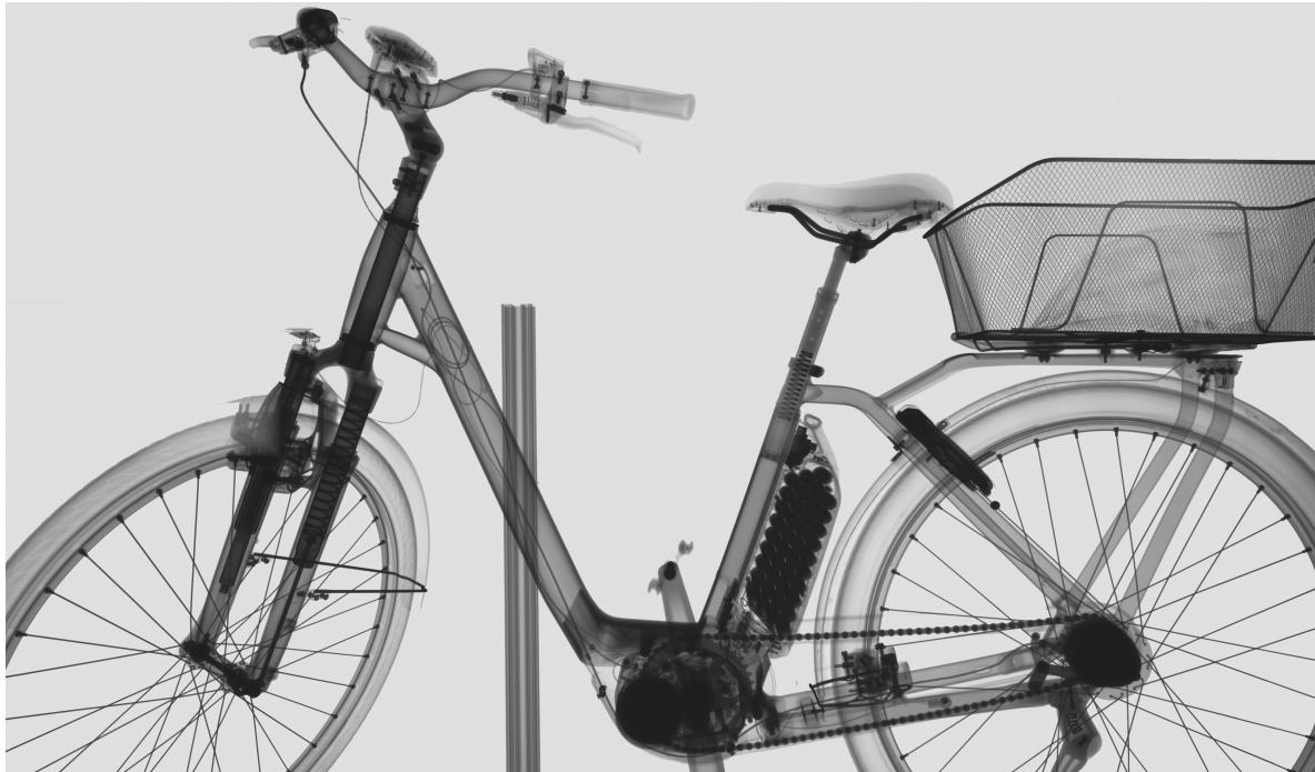
Figure 9. X-ray projection of a bike scanned at the Deggendorf Institute of Technology. A photograph of the robot CT system and the scanning progress is shown in Figure 1.
