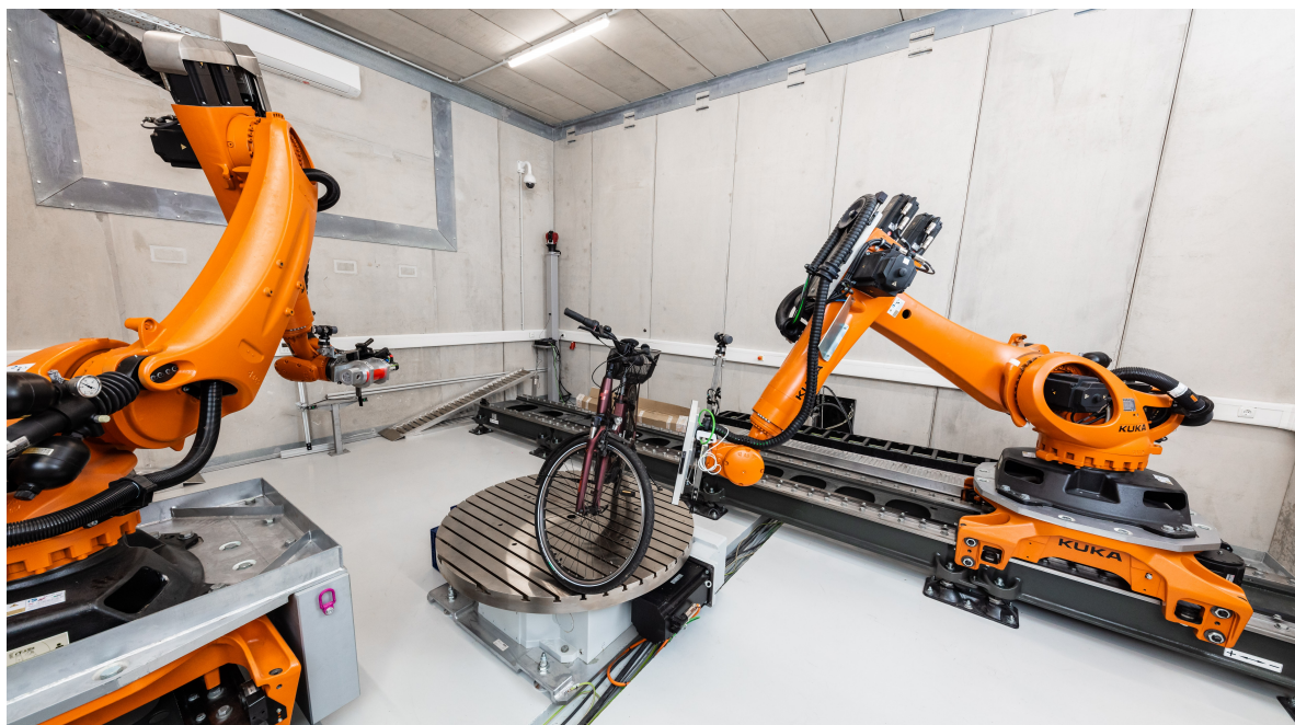
Figure 1. Twin robotic CT system at the Deggendorf Institute of Technology scanning a bike.
