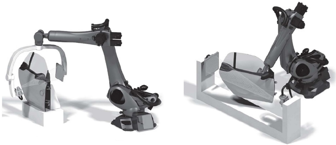
Figure 4. Sketch of two setups of industrial mono robotic CT systems scanning a car door [37].
