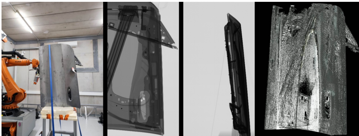
Figure 12. Robotic CT scan of a BMW car door conducted by the Deggendorf Institute of Technology. Left: Photograph of the mounted door. Middle: Two X-ray projections. Right: Rendering of the reconstructed CT volume (with some remaining metal artifacts) [14].
