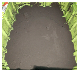
Figure 8. The photograph of the solid residue removed from the "dry" cyclone.
