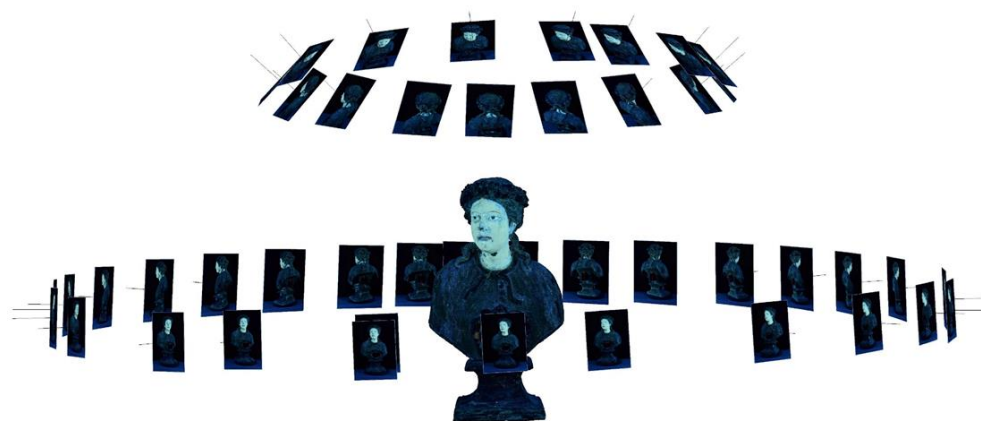
Figure 2. Creation of the 3D UVF model starting from the images acquired by rotating the object, in this case a reliquary bust representing St. Rosalia, and maintaining fixed the camera and the UV sources [42].
