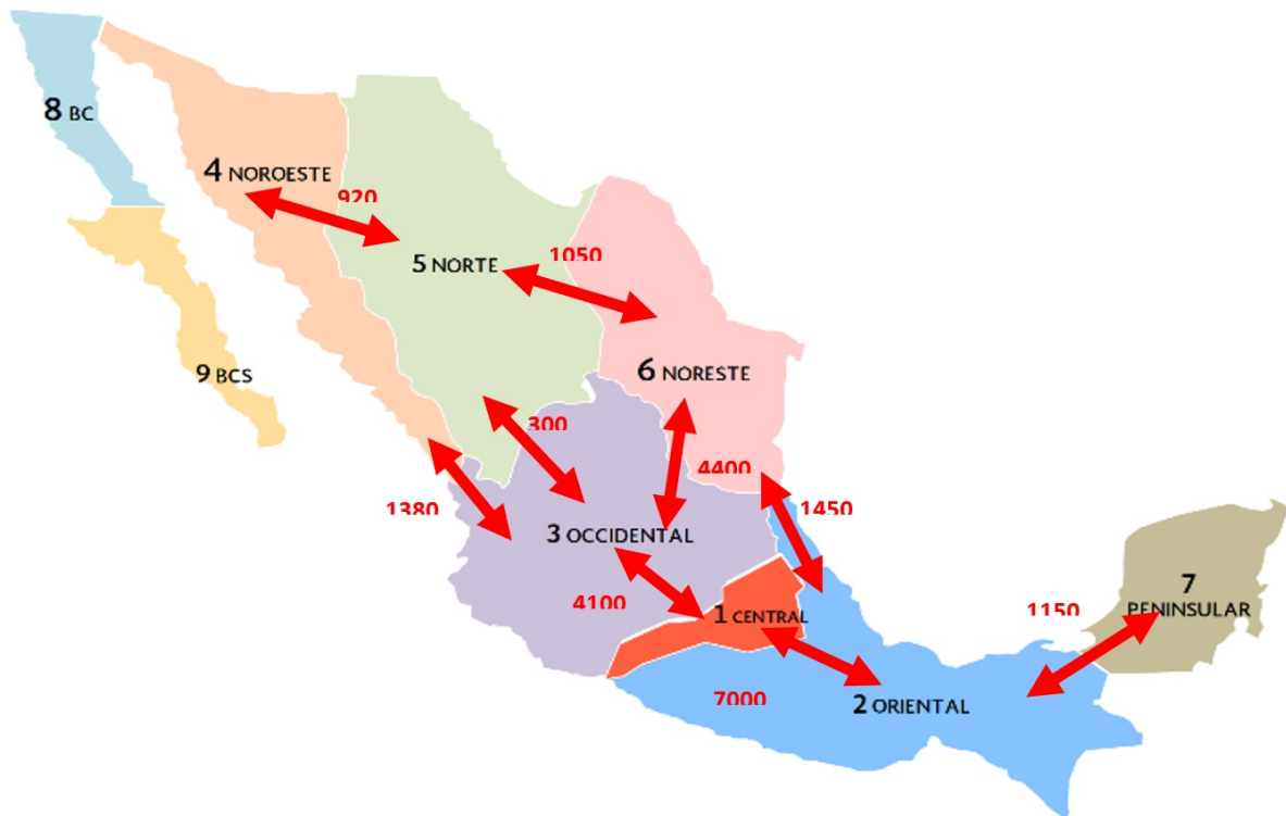
Figure 2. Capacity of the 9 transmission lines (MW) between the SEN's different generation and consumption regions.
