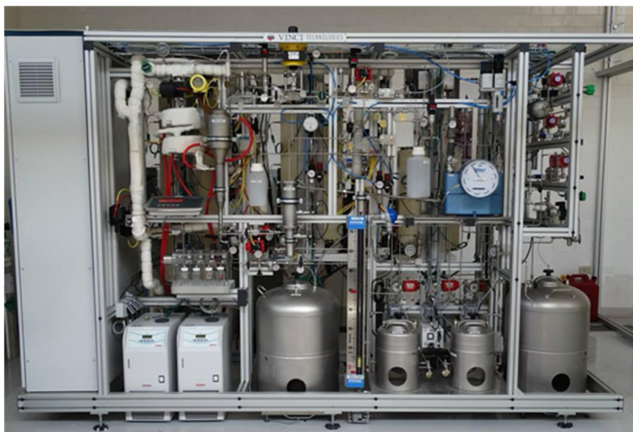
Figure 4. Semi regenerative pilot plant of the NCR process.
