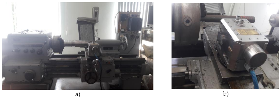
Figure 4. Appearance of the experimental setup: a) 1K625 machine tool, b) measuring unit STD.201-1.
