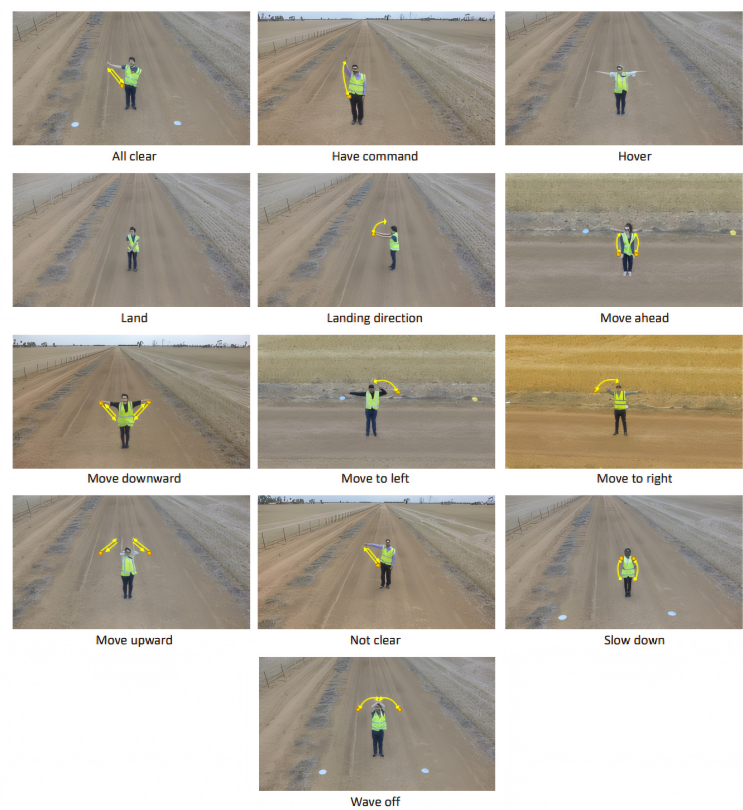
Figure A14. This diagram displays thirteen explicitly chosen gestures, each accompanied by a single picked image. Directions of hand movement are shown by the arrows. The amber color marks serve as approximate indicators of the initial and final locations of the palm for ONE iteration. Neither the Hover nor Land gestures are dynamic gestures.
