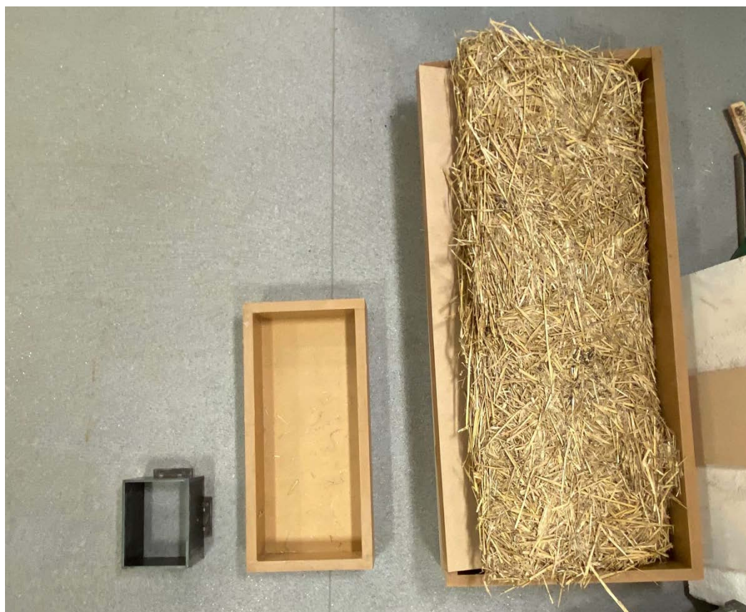
Figure 4. The 3 moulds used to produce the sample wheat straw panels.
