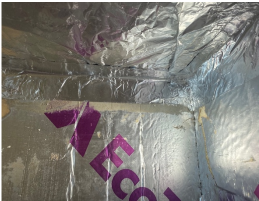
Figure 6. The hotbox interior and the wheat straw panel with heat flux sensor.
