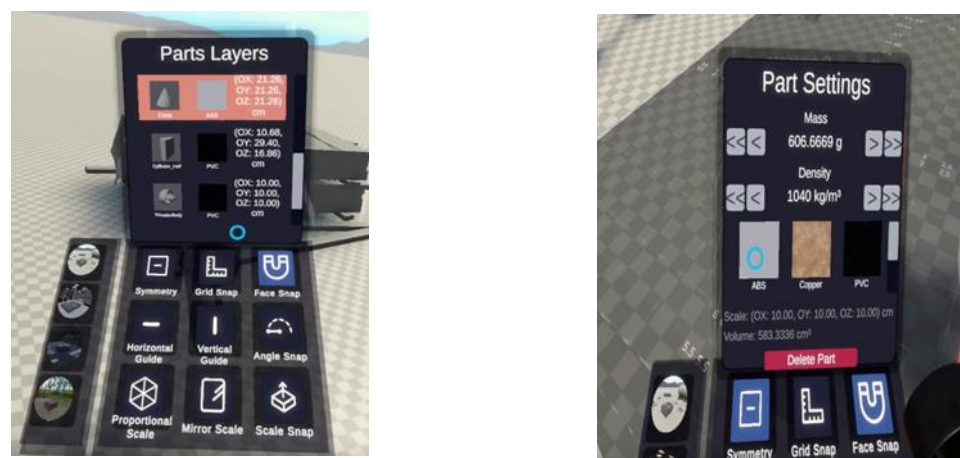
a. Viewing mode for individual b. Setting the mass, density and material for a specific shapes contained in the model shape contained in the model
