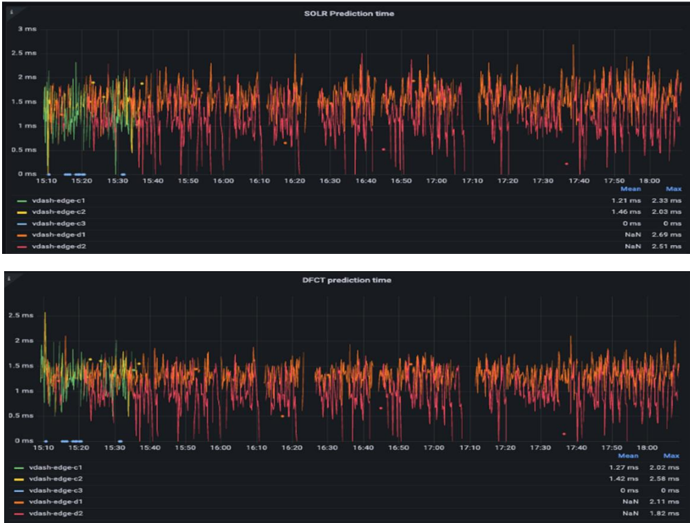
Figure 20. (top) Processing time of the defects detection algorithm, (bottom) processing time of the corrosion detection algorithm. Both running in parallel on the same images.
