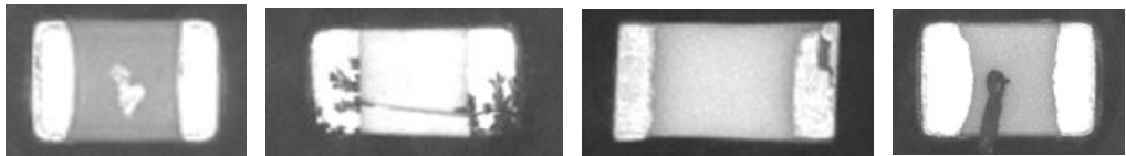
Figure 1. Examples on Passive Components (Left to Right): Conductive FOD (Foreign Object Debris), Corrosion leading to cracks, Leads peeling, Non-conductive FOD.
