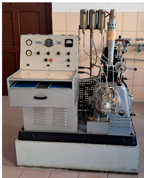
Figure 1. Test rig for measuring the cetane number of diesel fuel
