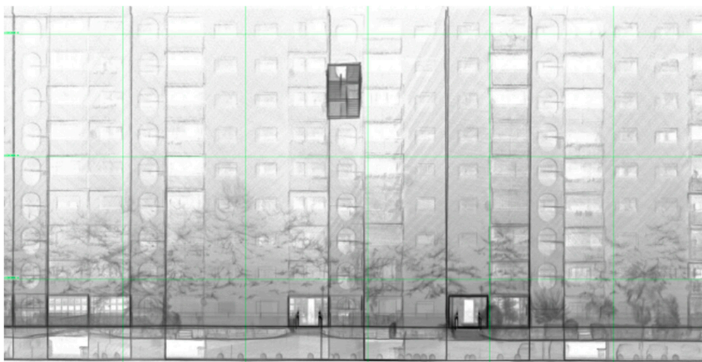
Figure 25. An example of one of orthophoto views of the facades of the buildings requested in the Milan project. The survey is carried on with Terrestrial Laser scanner, without use of control points, at the nominal scale of 1:200
