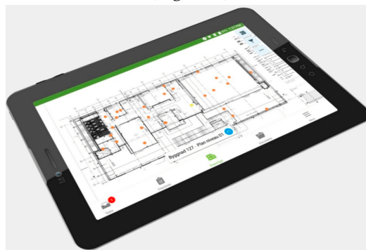
Figure 4. The use of a tablet with a floor plan on the background is currently use for census projects. Courtesy of Dalux [82].
