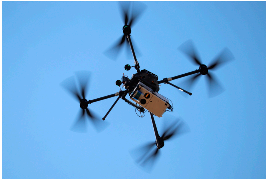
Figure 2. UAS flying the payload of a hyperspectral imager (Mjolnir VS-620) and Lidar.
