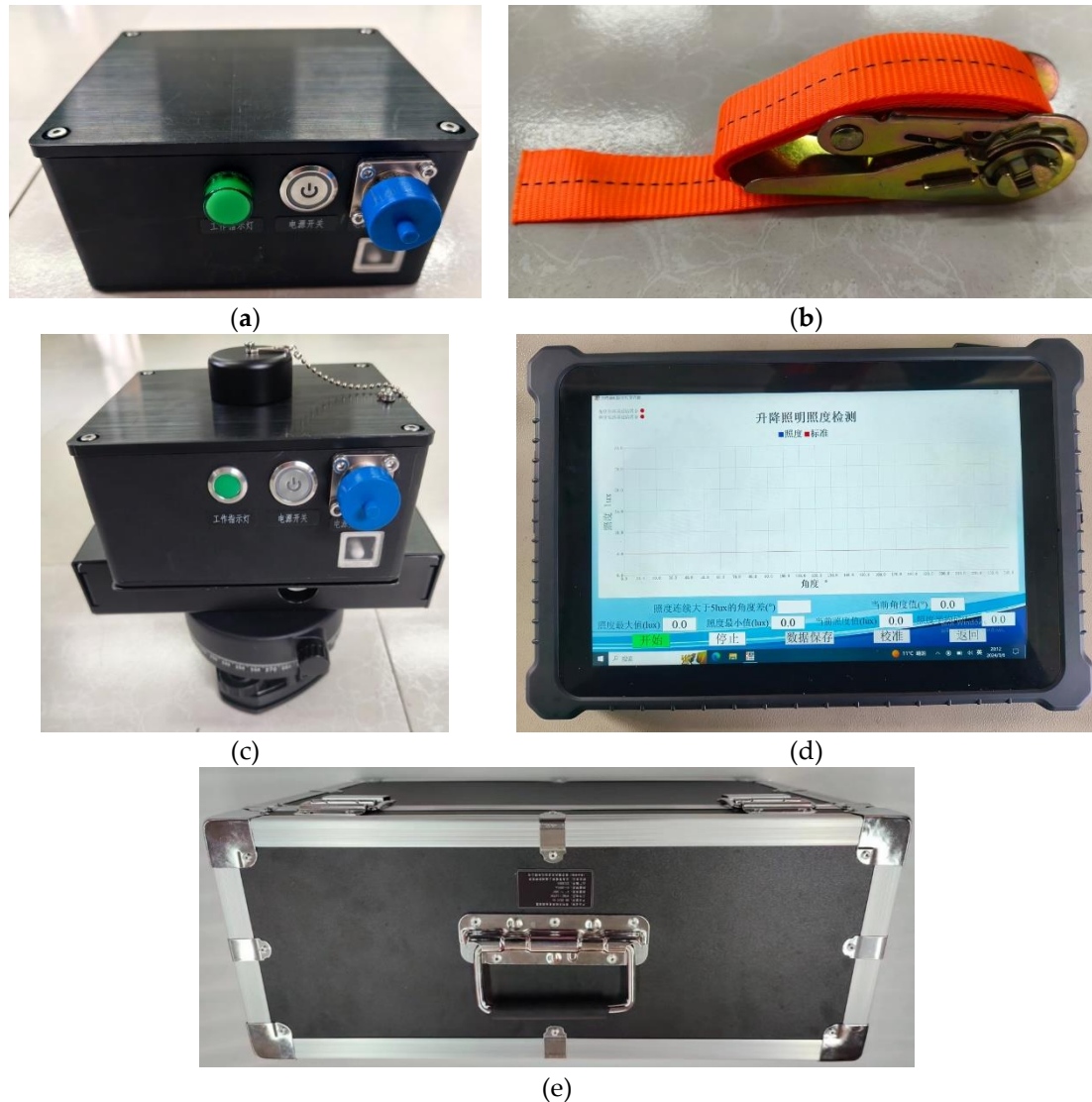
Figure 8. Physical diagram of the entire testing device. (a) Angle detection device. (b) Ratchet tensioner. (c) Illuminance detection device. (d) Data integration terminal. (e) Toolbox for detection device.
