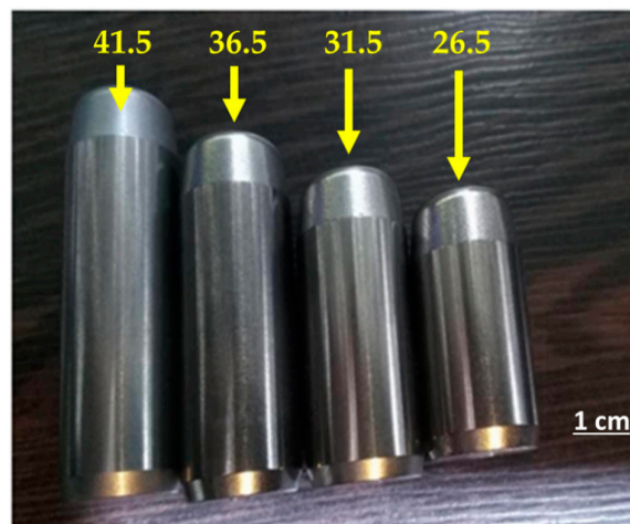
Figure 9. Sizes of replaceable studs: 26.5, 31.5, 36.5, 41.5.
