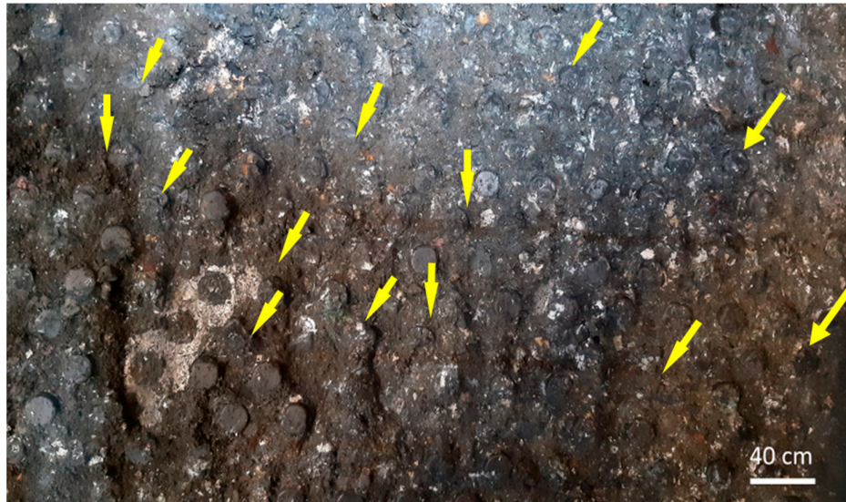
Figure 10. Failure to replace broken studs and continuation of the crushing operation.
