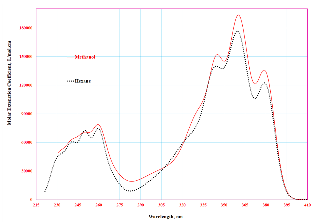
Figure 17. Electronic absorption spectrum of 4-benzylidene-2-phenyl-5(4H)-oxazolone in methanol and n-hexane.
