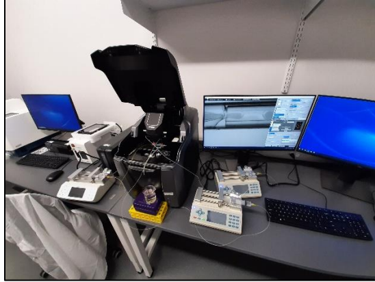
Figure S.3. Experimental setup for microsphere fabrication, showing the microscope and the three pumps for the sensing solution, PDMS, and PVA.
