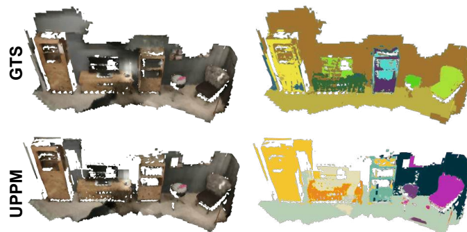
Figure 6. Qualitative comparison on the RIO dataset [54]. Top: Ground-truth panoptic segmentation and corresponding 3D map. Bottom: UPPM output with sharper object boundaries and more coherent semantic regions in cluttered, real-world scenes.
