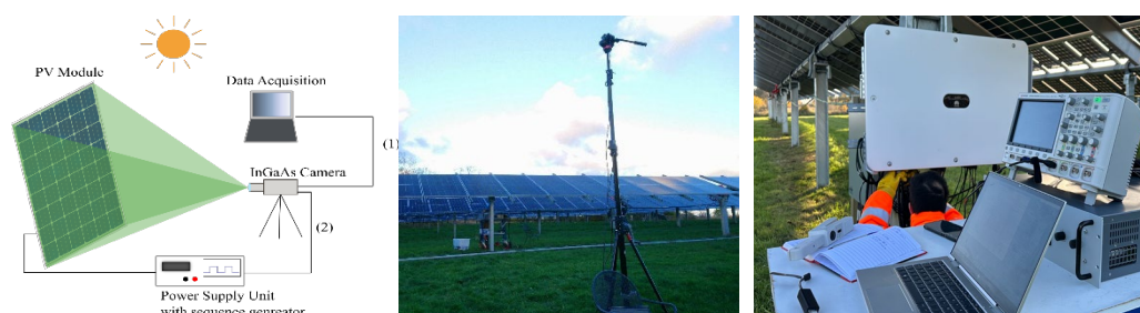
Figure 7. Schematic representation of a daylight EL imaging setup for PV modules.
