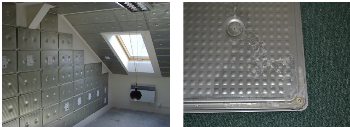
Figure 1. PCM encapsulated in aluminium container: (left) Experimental installation in the test room; (right) PCM leakage on the surface of aluminium container.
