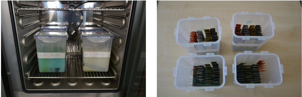
Figure 8. Metal samples prepared for corrosion testing: (left) Test beakers placed in environmental chamber; (right) Samples in test beakers.
