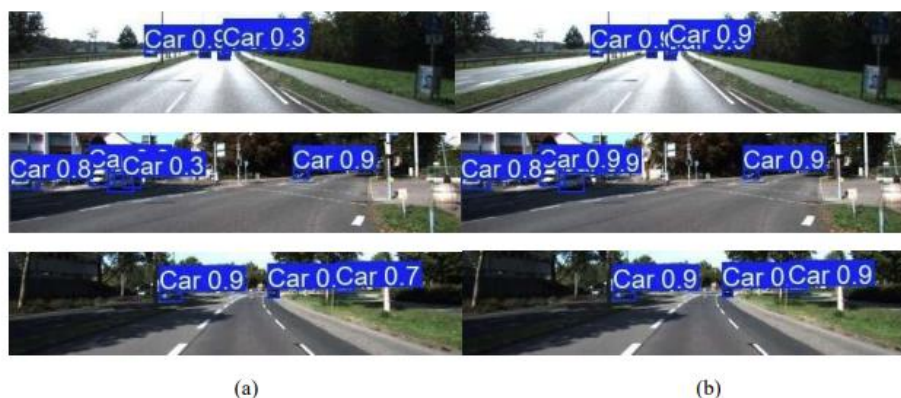
Figure 8. Visualization analysis of the experimental results.(a) Images detected by YOLOv8 (b) Images detected by SST-YOLO.
