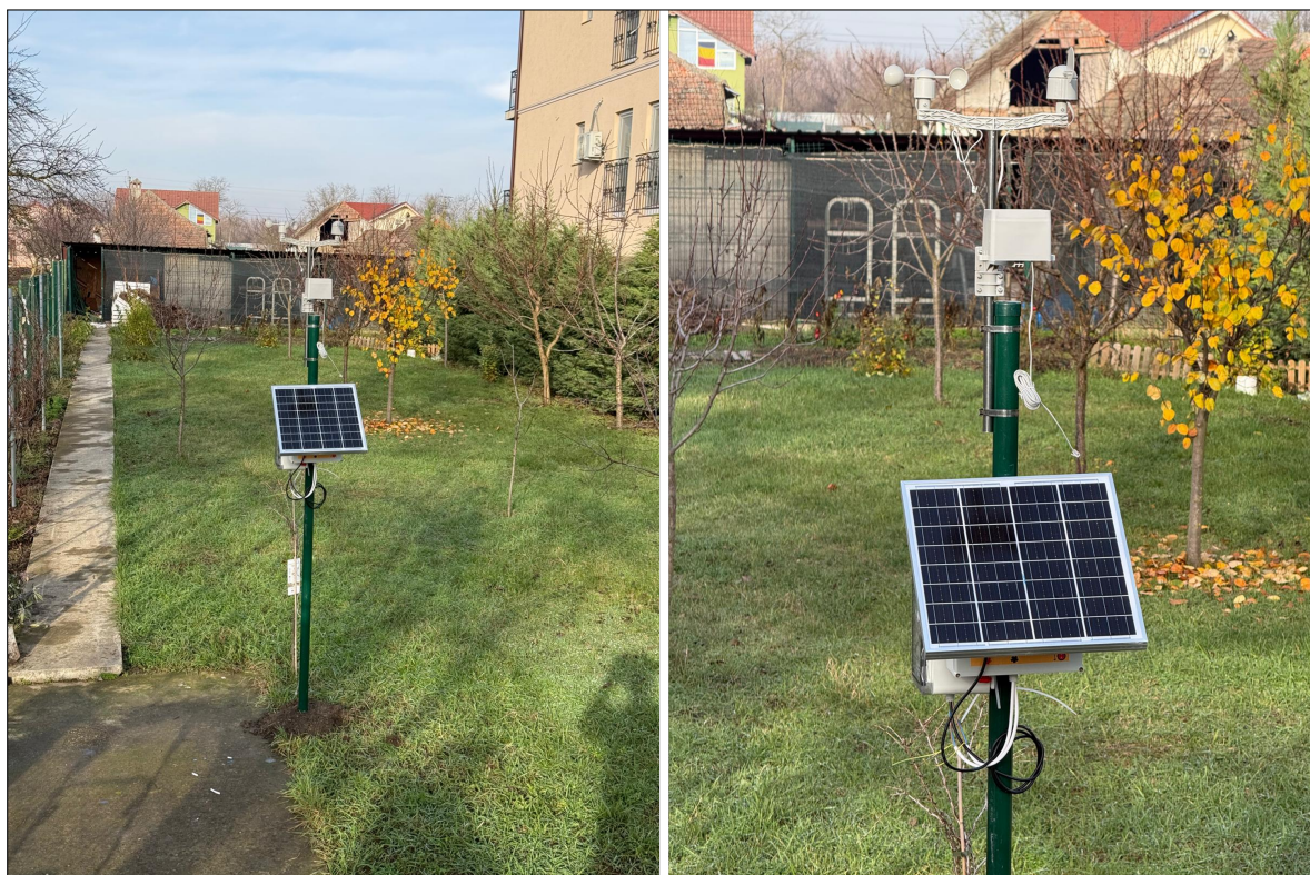
Figure 2. Field deployment of the proposed solar-powered environmental monitoring platform in Sânnandrei, Timiș County. The installation illustrates real-world integration of the sensing platform within an agricultural environment characterized by stable LTE-M network coverage.
