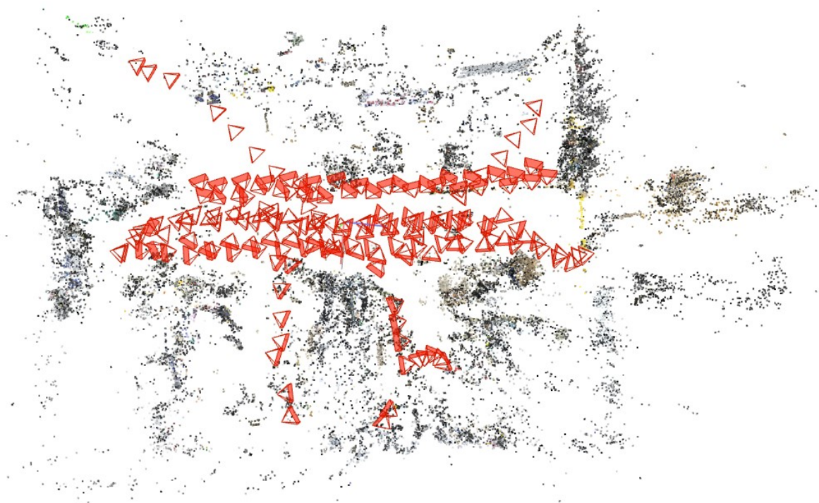
Figure 6. Lab point cloud and camera poses generated by ORB-SLAM for 3DGS optimization.
