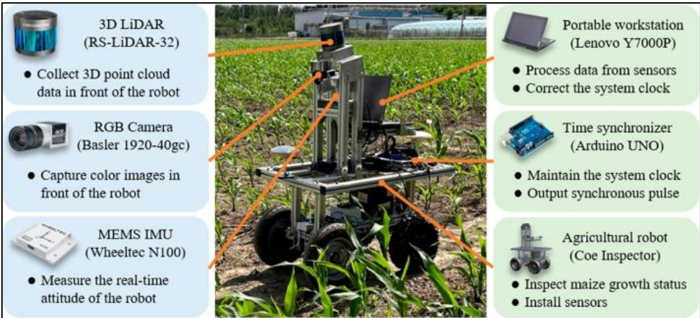
Figure 2. Multiple sensor device developed by Ban et al. Adapted from [29], © 2024, licensed under CC BY-NC-ND.
