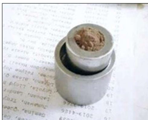
Figure B.2.2.1. Placing 4 grams of pulverized aged sample into the pelletizer.
