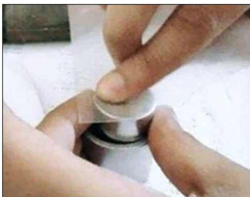
Figure B.2.2.2. Pressing and compacting by the pelletizer.
