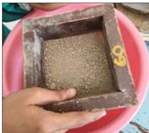
Figure B.1.2. Clay sample preparation: 60-mesh sieving.
