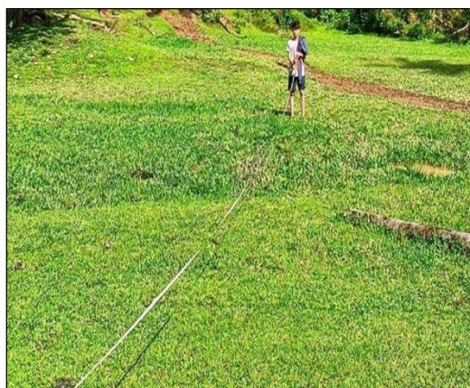
Figure A.1.1 Performing Composite Sampling Method (zigzag pattern), 10 sampling points with a regular interval of 10 meters.
