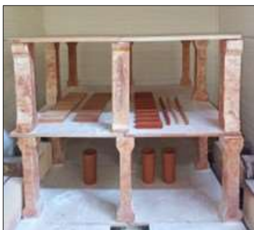
Figure B.2.3.2. Kiln Firing of Test bars and Pellets.
