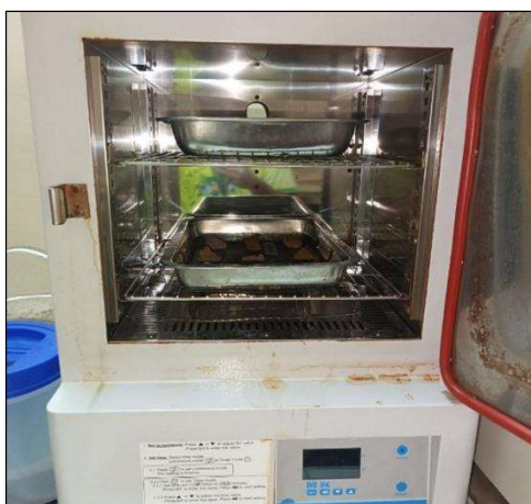
Figure B.2.3.1. Test bars and Pellets Oven Drying at 110° C of temperature.
