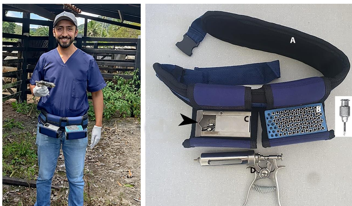
Figure 4. On the right, a device for single-use needles and their reuse after disinfection. Belt (A) with a needle holder with 91 disinfected needles ready for use (B) and a container (C) for the needles after use. This container has an angled edge (arrow) that aids in removing the needle from the syringe (D). On the left, the arrangement of the equipment on the person vaccinating the cattle.
