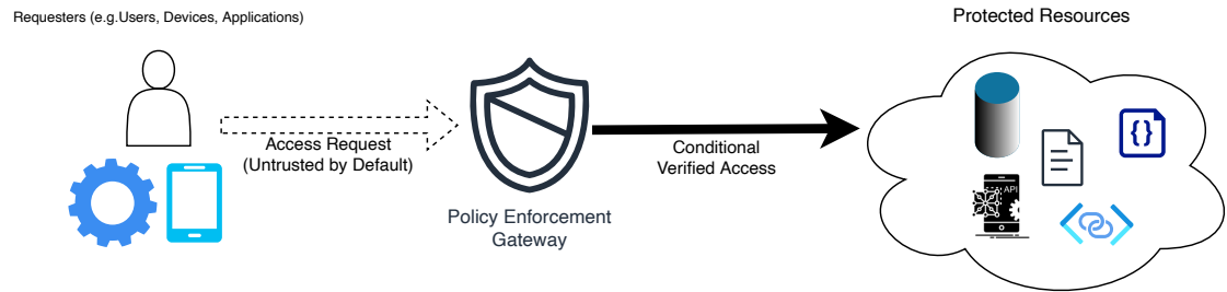
Figure 4. NIST ZT General Idea. This image has been completely re-modified; however, the idea of the image was inspired by [39,46]
