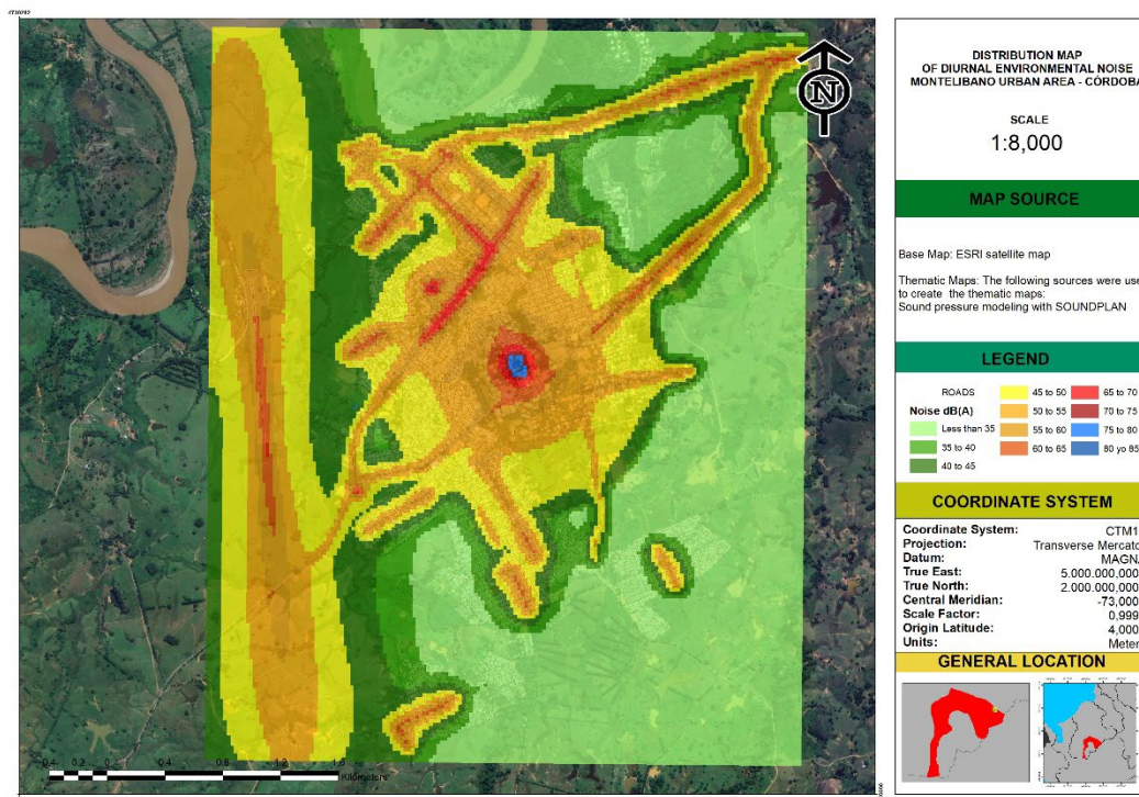
Figure 7. Modelled Environmental noise distribution in Montelíbano — diurnal scenario. Environmental noise integrates vehicle, industrial, commercial and residual anthropogenic sources. The high-energy concentration at the central commercial area (65–70 dB(A)) and along the corridors is consistent with the vehicular pattern, while the airport-trajectory corridor (left edge) introduces an additional aeronautical contribution.
