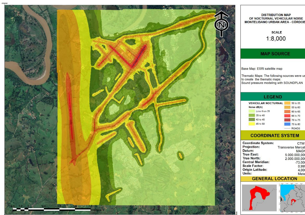
Figure 6. Modelled vehicular noise distribution in Montelíbano — nocturnal scenario. Despite the regulatory threshold reduction (75 to 70 dB(A) industrial; 70 to 55 dB(A) residential), the spatial pattern preserves the same hot-spots as the diurnal scenario, in clear contrast with the strong day–night contraction observed in Soledad (cf. Figures 1–2).
