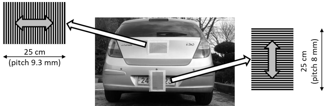
Figure 29. Layout of simultaneous horizontal and vertical measurements. The direction of measured vibration is indicated on each grid by a thick double-headed arrow.
