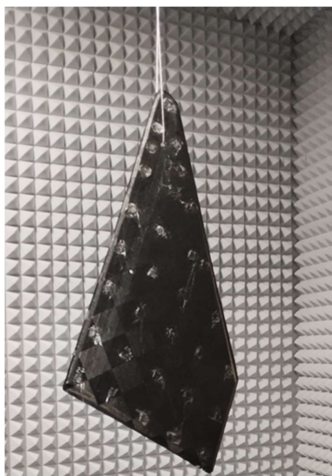
Figure 6. Free–free suspension of the winglet using elastic cords.
