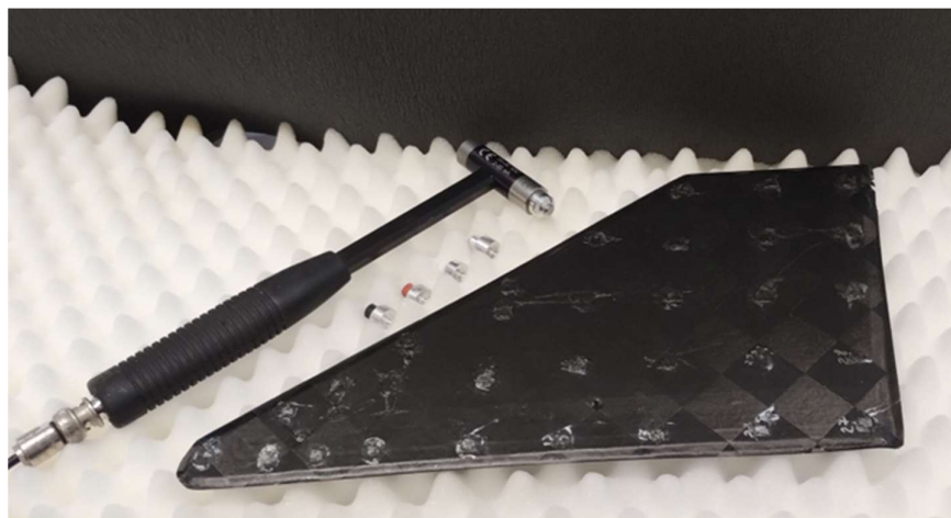
Figure 7. Winglet supported on a soft prismatic foam, with modal hammer with interchangeable impact tips.
