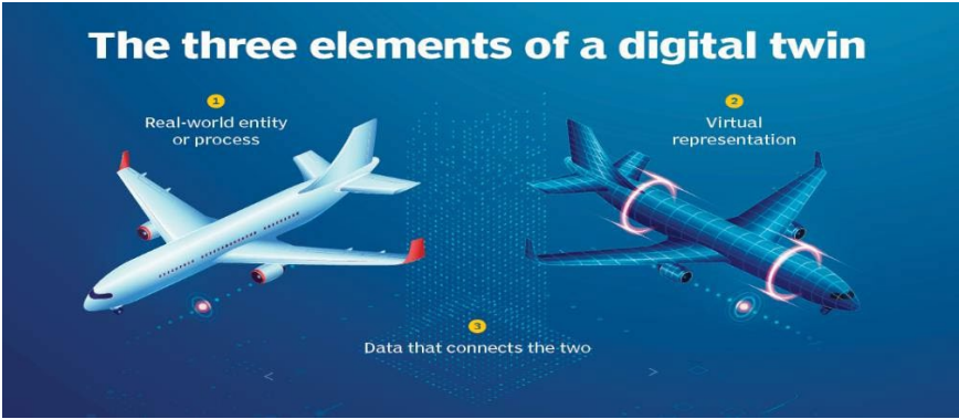
Figure 3. Component of Digital twin technology: 1. Physical entity, 2. Virtual entity, 3. Data connection between Physical & Virtual entities (Mary E. Shacklett, 2025).
