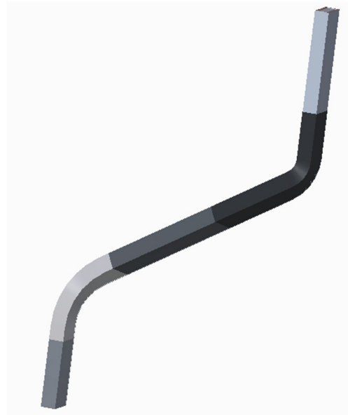
Figure 4. Anti-corona stator bar structure.
