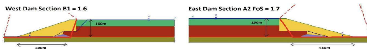
Figure 1. Morgenstern-Price computed FoS for 2D models of cross sections based on 2020 KCB stability analyses and minimal slip surfaces [Tetra Tech, 2021].
