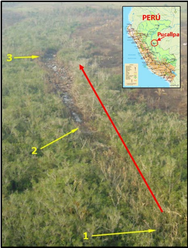
Figure 2. Aircraft impact location - A.A.H.H. La Florida - Pucallpa [6]. The impact path is highlighted in red, while the beginning of contact with the trees is indicated with a yellow indicator (1) and the point of impact of the front part of the fuselage with another yellow indicator (2). The final position of the wreckage of the aircraft and the location of the fire are indicated by a third yellow indicator (3).
