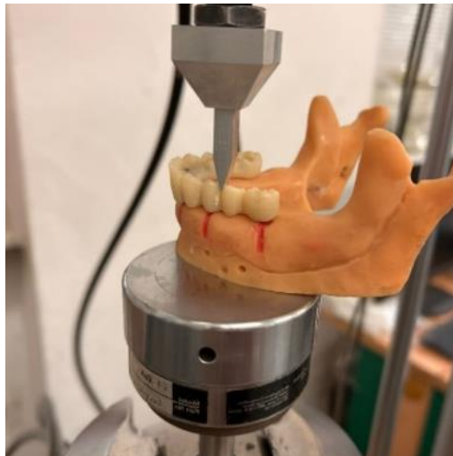
Figure 6. Model gripped onto the MTS 858 machine during cyclic tests.
