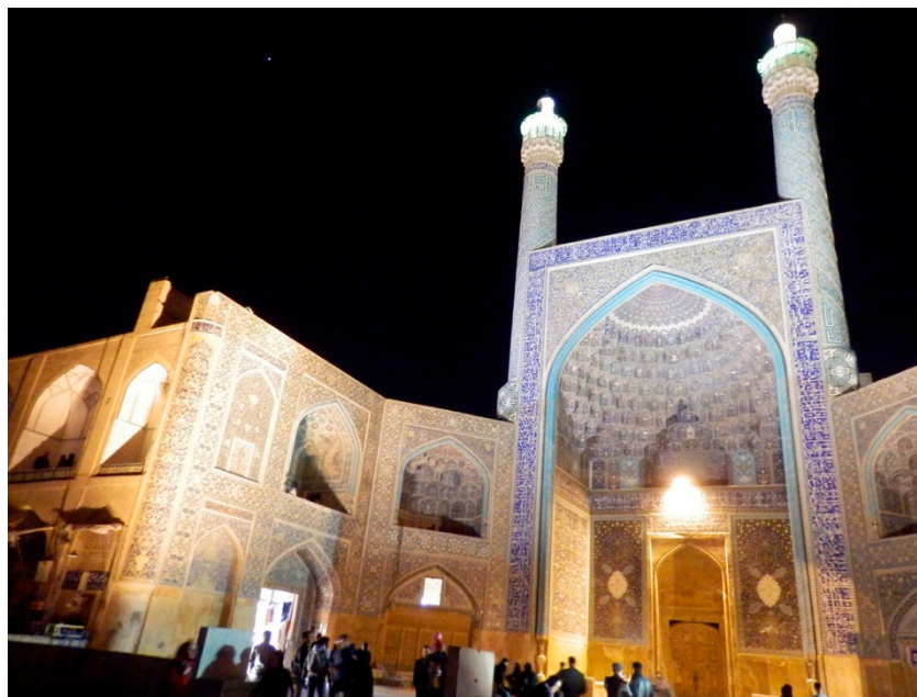
Figure 6. Pure floodlighting without layering of light diminishes the details and special characters of Islamic architecture of the Royal Mosque entrance at the Naghshe-Jahan-Square site.
