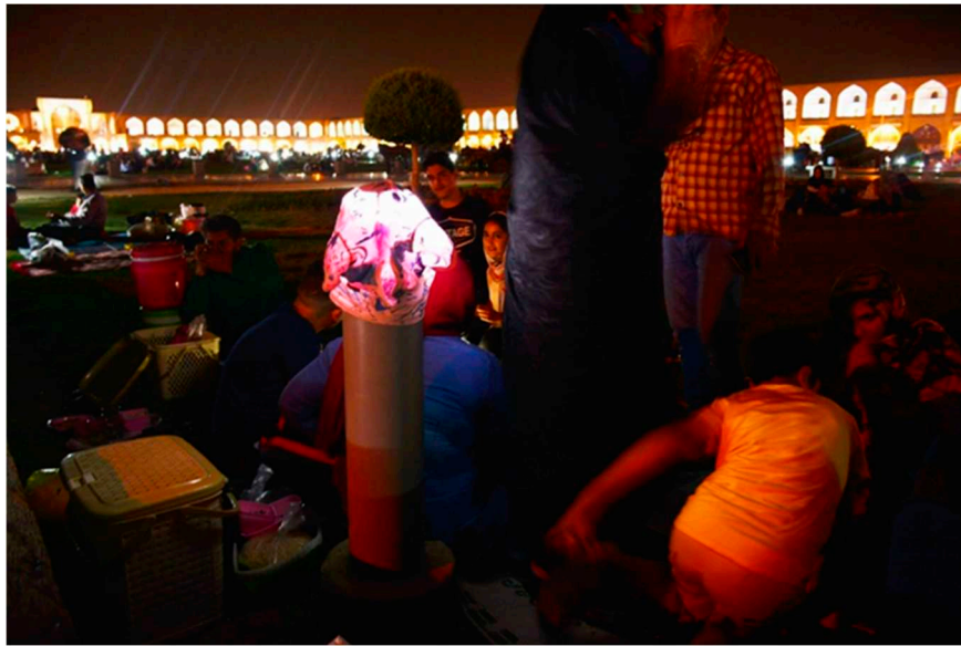
Figure 7. A piece of cloth is used to cover the luminaire for reducing glare at the Naghshe-Jahan-Square site.
