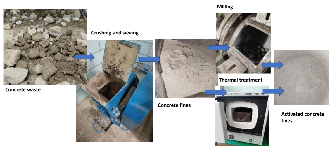
Figure 2. Manufacturing the recycled concrete fines in the lab: crushing the concrete rubble in a jaw crusher; sieving and milling in the ball mill (mechanical activation).
