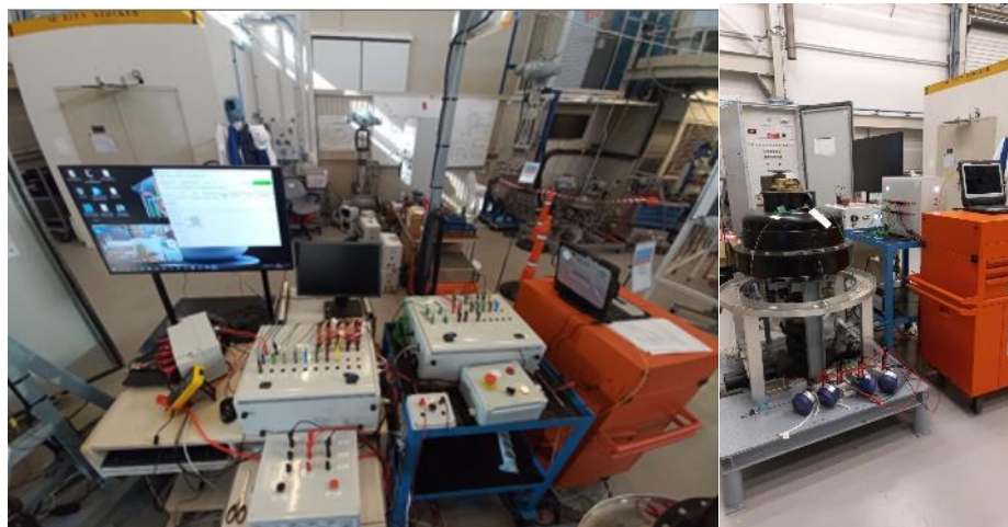
Figure 12. Test bed on real sensors and actuators at EDF R&D "valves laboratory" facility.
