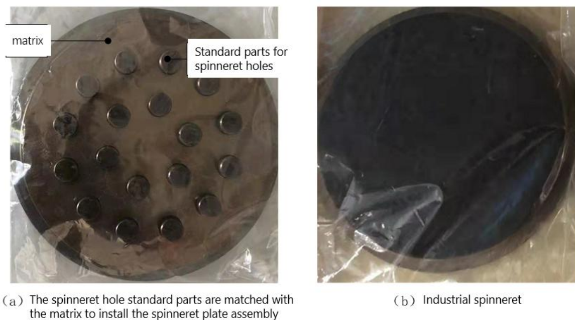
Fig. 2 Comparison between the industrial spinneret and spinneret assembly designed in this paper
