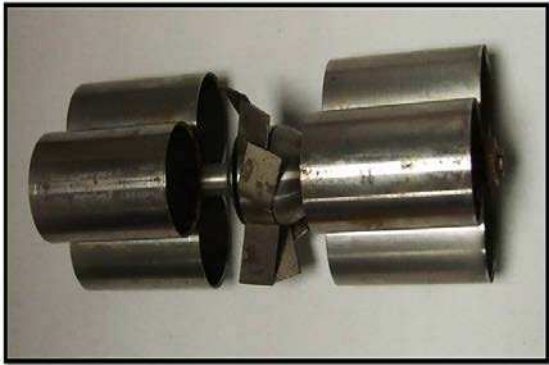
Figure 3. Turbine meter with damaged blades in Cavitation-Induced Flows.
