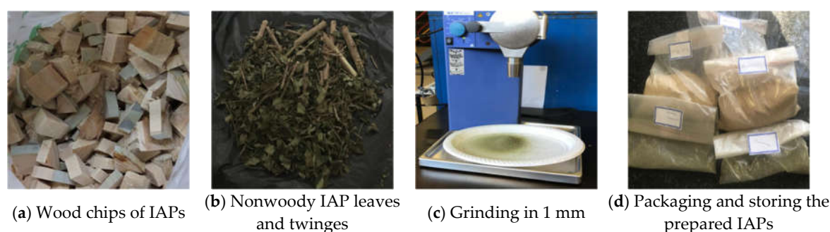
Figure 1. Stages of preparation for woody and nonwoody IAPs for analysis.
