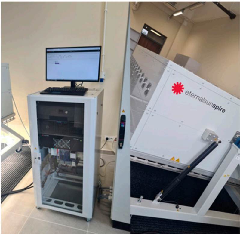
Figure 1. Large-scale steady-state stationary solar simulator, class AAA.
