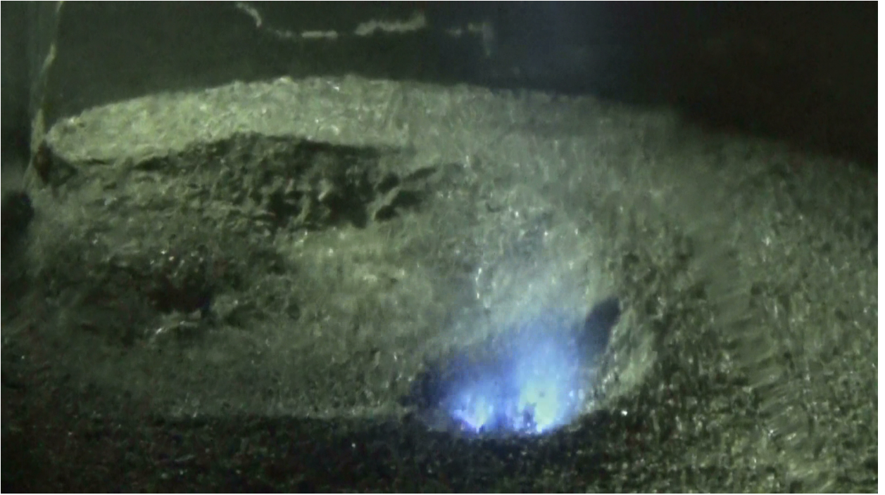
Figure 10: Dynamic EDM crater formation. The end result of the crater in Fig 9. When the discharge finally became stagnant, the end result was a straight edge crater with a smaller crater perched on the larger crater wall. As noted in section 1.2, this feature is more common than what can be considered random and was a frequent result of EDM experiments.
