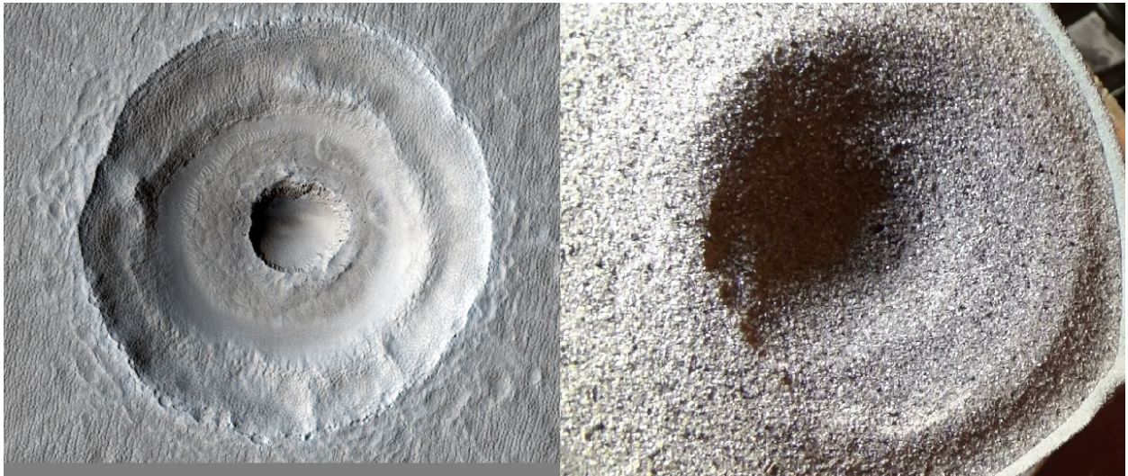
Figure 13: Multiple walls comparison. Left: a crater from the Arcadia Planitia region, Mars, with multiple walls forming three concentric rings. Right: an EDM crater with several walls that formed by repeated collapsing and machining. Credit: NASA/JPL/University of Arizona.
