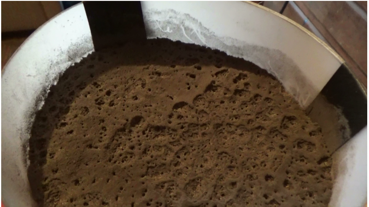
Figure 1: Pinhole channels. Pinhole sized channels form as a result of outgassing due to low atmospheric pressures. Outgassing may explain the observation of high porosity associated with low pressure bodies. If so, this would suggest a sudden loss of atmosphere in those bodies.
