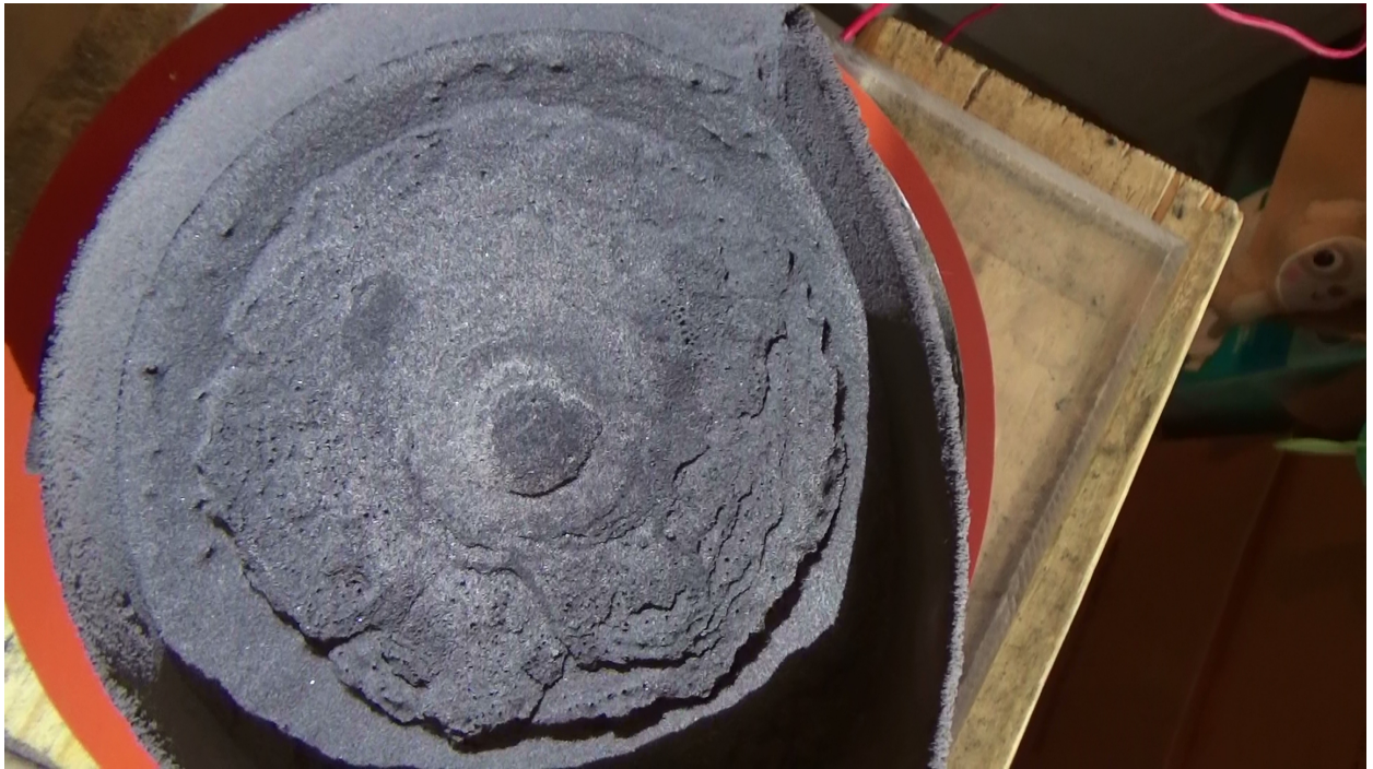
Figure 3: EDM crater, fine material. Collapsing and terracing are a common feature of craters, resulting from gravitational slumping of material at the crater wall.
