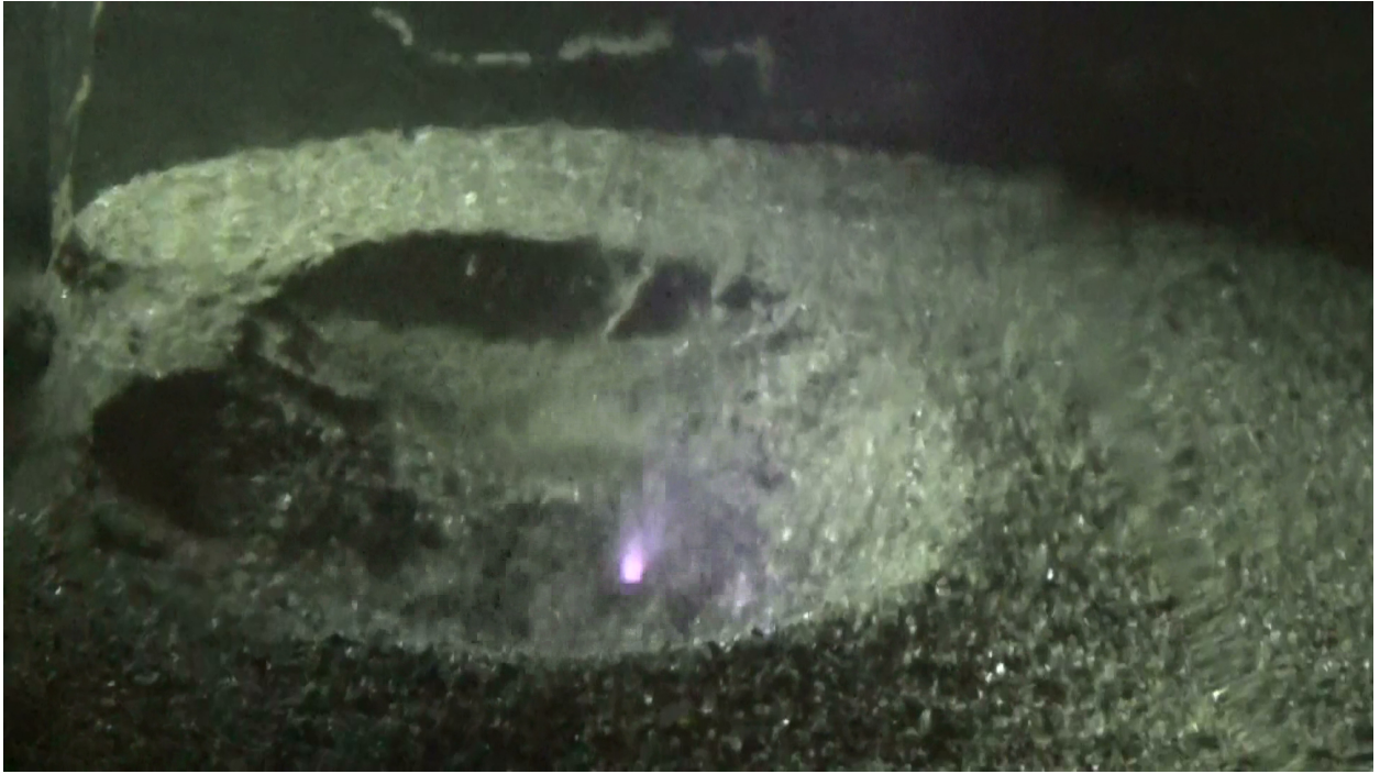
Figure 9: Dynamic EDM crater formation. This crater formed as a pair of craters throughout the discharge, changing in shape and size for roughly 10 minutes. Here we observe a proverbial heart shape that can also be found on celestial bodies.
