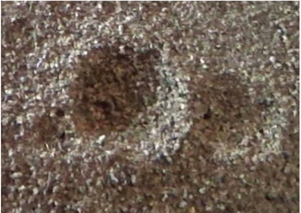
Figure 7: Three EDM craters sharing walls. A close up of three craters that formed in a field and share walls. The largest of them having a roughly 1 cm diameter.
