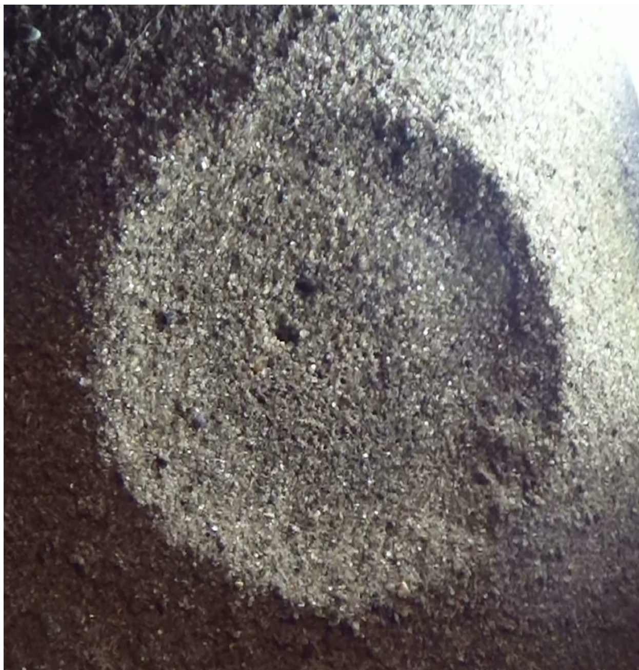
Figure 5: Small EDM crater. A small crater with a broad flat floor and ridges. Center left of the crater: larger channels are visible where the discharge became stagnant before being terminated.
