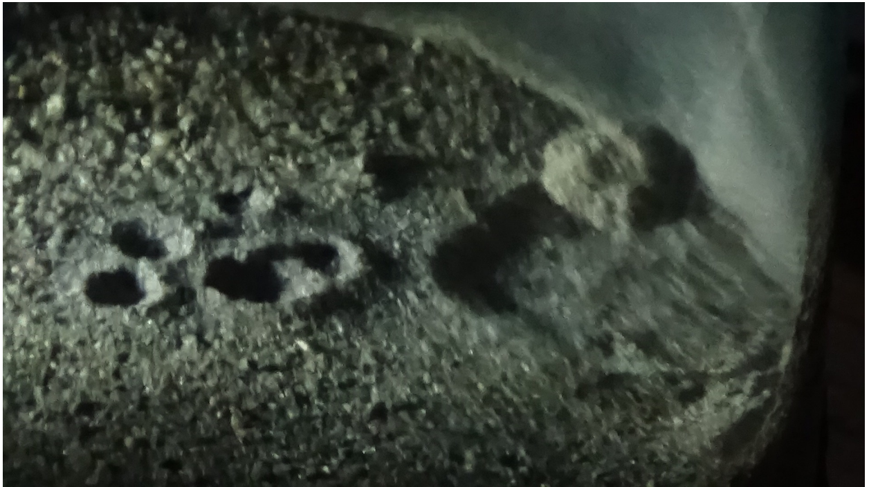
Figure 6: EDM crater field. A field of six craters of varying size, some sharing rims. It would be suspected these fields occur as a result of changing potentials at the surface, the discharge consequently taking the path of least resistance and forming several craters in the process.
