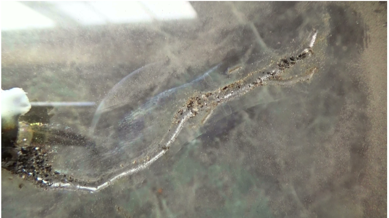
Figure 14: Sinuous rille in acrylic. A sinuous rille melted into the bottom of the acrylic chamber that housed the experiment. To the left of the image (not visible) is the cathode.
