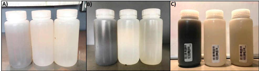
Figure 2. Samples from storm events of varying intensities at the 3 sampling sites. A) Low intensity storm (~1.3-mm/hr, or 0.05-in/hr), B) Medium intensity storm (~3.8-mm/hr, or 0.15-in/hr), and C) High intensity storm (~10.2-mm/hr, or 0.40-in/hr). In each photo the bottles, from left to right, are: control, porous asphalt overlay, and full-depth porous asphalt.
