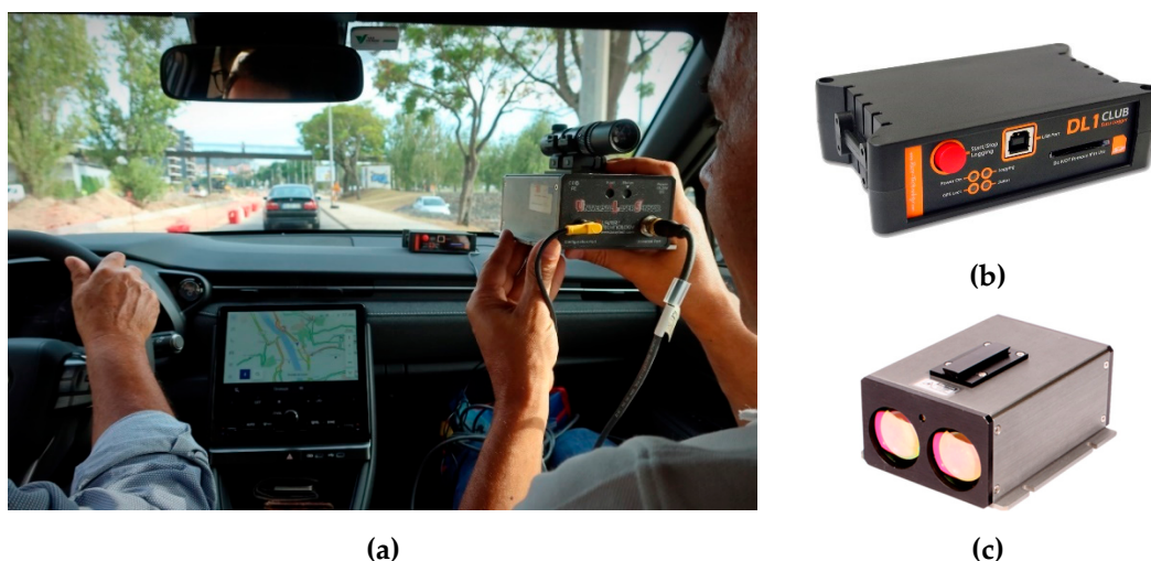
Figure 1. Data acquisition system. (a): Installed equipment and leader–follower vehicles; (b) datalogger; (c) Lidar sensor.
